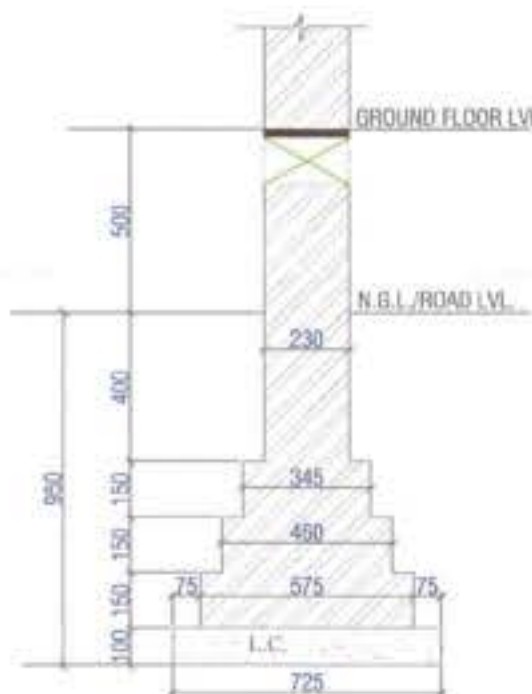
TYP. SECTION FOR 230 THK. BRICK WALL (scale: 1:20)
