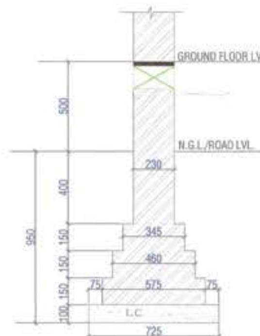
TYP. SECTION FOR 230 THK. BRICK WALL (Scale=1:20)
