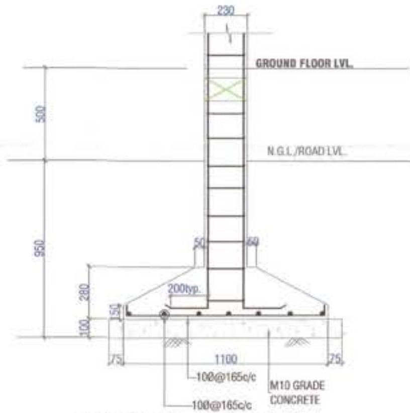
TYP. SECTION OF COLUMN FOOTING (scale:1:20)
