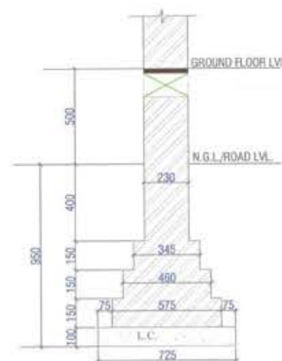
TYP. SECTION FOR 230 THK. BRICK WALL (Scale=1:20)
