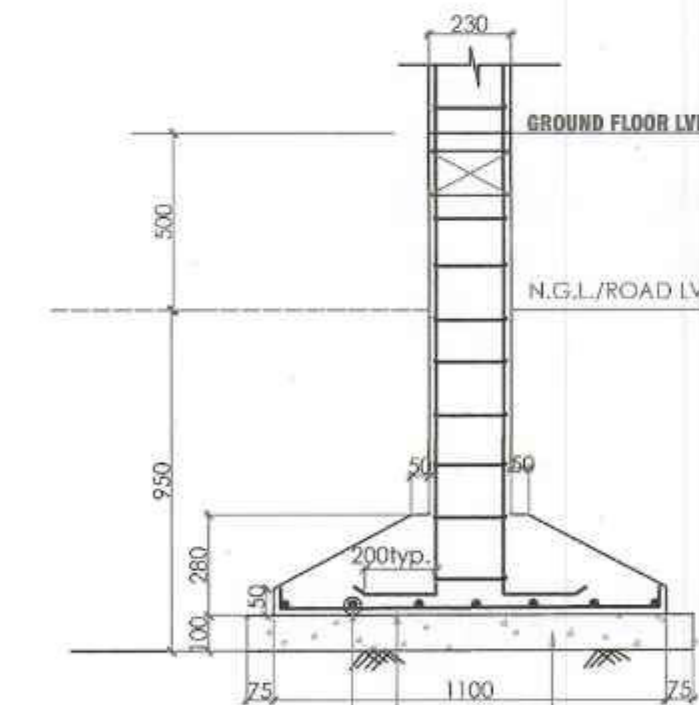
TYP. SECTION OF COLUMN FOOTING (scale=1:20)
