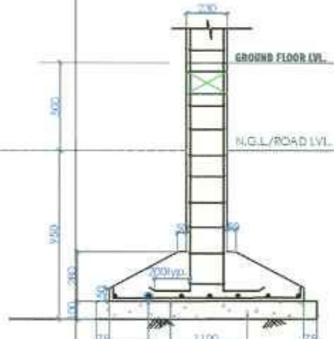
TYP. SECTION OF COLUMN FOOTING (Scale=1:20)
