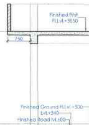
TYP. SECTION FOR 230 THK. BRICK WALL (scale=1:20)
