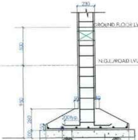
TYP. SECTION OF COLUMN FOOTING (scale=1:20)
