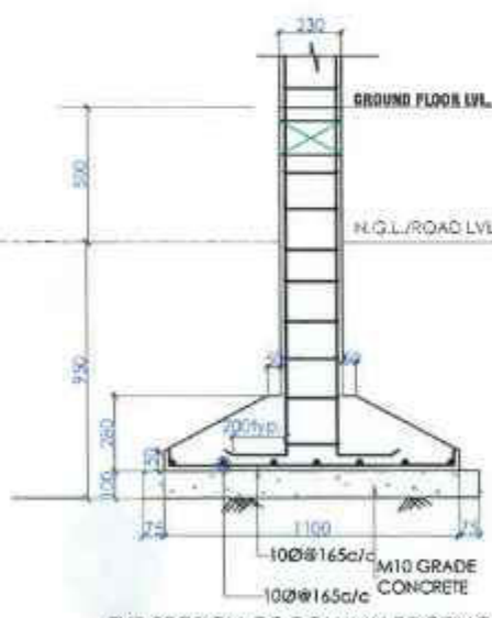
TYP. SECTION OF COLUMN FOOTING (scale=1:20)
