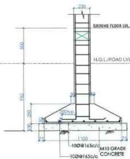
TYP. SECTION OF COLUMN FOOTING (scale=1:20)
