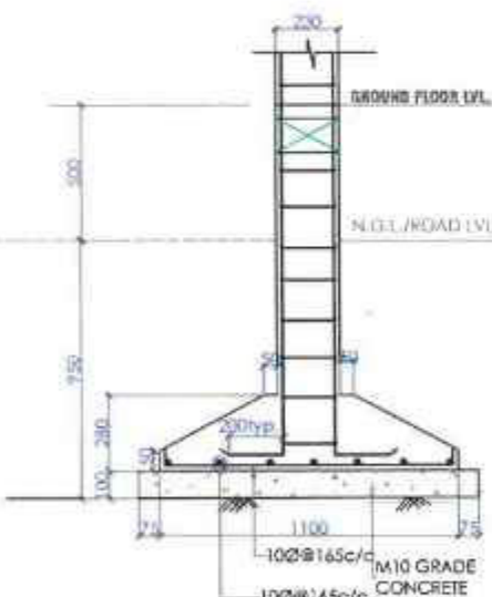
TYP. SECTION OF COLUMN FOOTING (scale=1:20)
