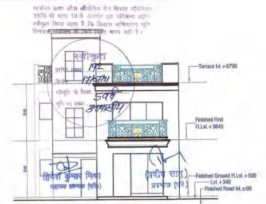
FRONT ELEVATION (SCALE=1:100)
