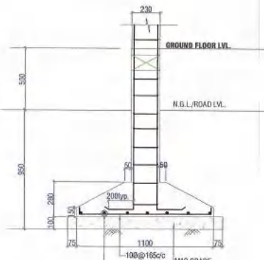
TYP. SECTION OF COLUMN FOOTING (Scale=1:20)
