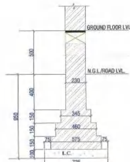
TYP. SECTION FOR 230 THK. BRICK WALL (Scale=1:20)
