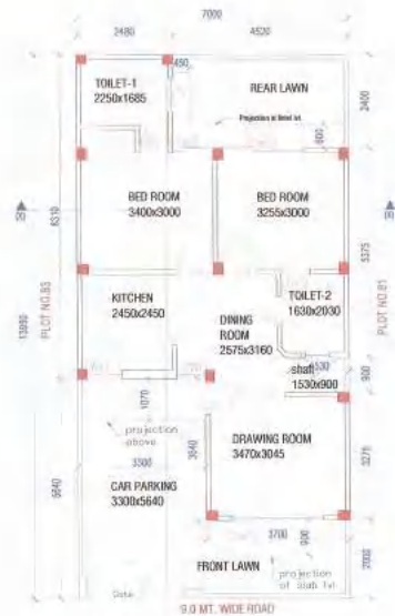
GROUND FLOOR PLAN (SCALE=1:100)
