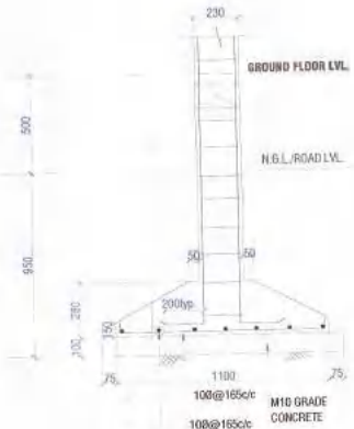
TYP. SECTION OF COLUMN FOOTING (SCALE=1:20)
