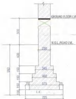
TYP. SECTION FOR 230 THK. BRICK WALL (Scale=1:20)
