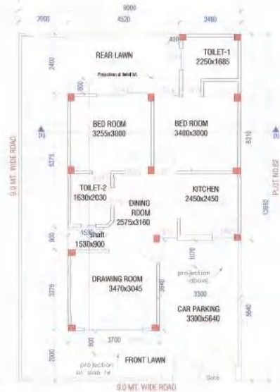
GROUND FLOOR PLAN (SCALE=1:100)
