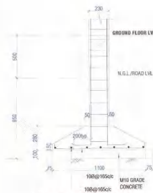
TYP. SECTION OF COLUMN FOOTING (Scale=1:20)
