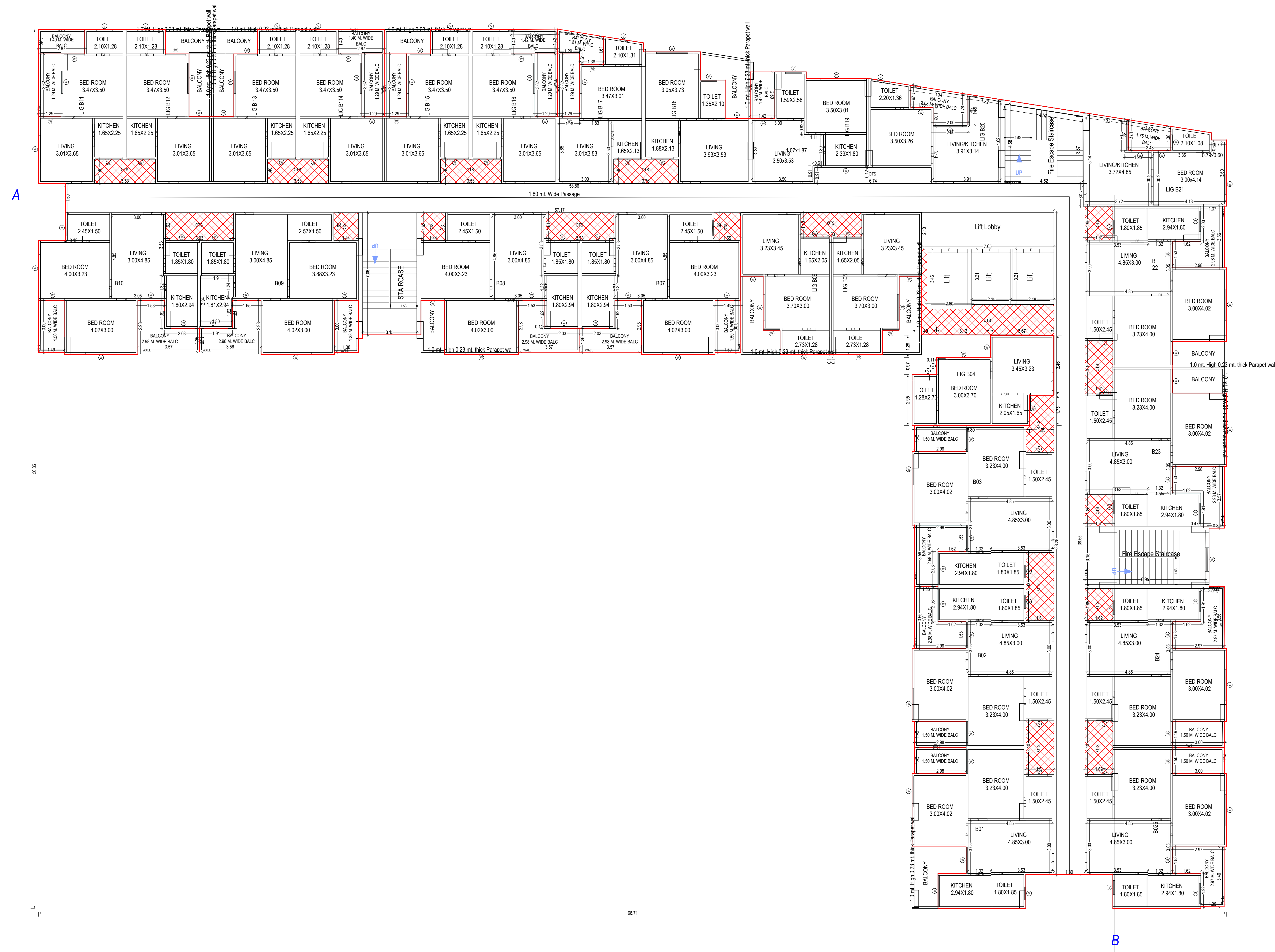
TYPICAL - 1, 2, 3, 4, 5, 6, 7, 8 FLOOR PLAN (Proposed) (SCALE 1:100)
