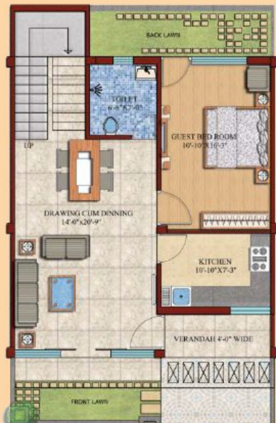
GROUND FLOOR PLAN (COVER AREA 855.66 SQ.FT)
