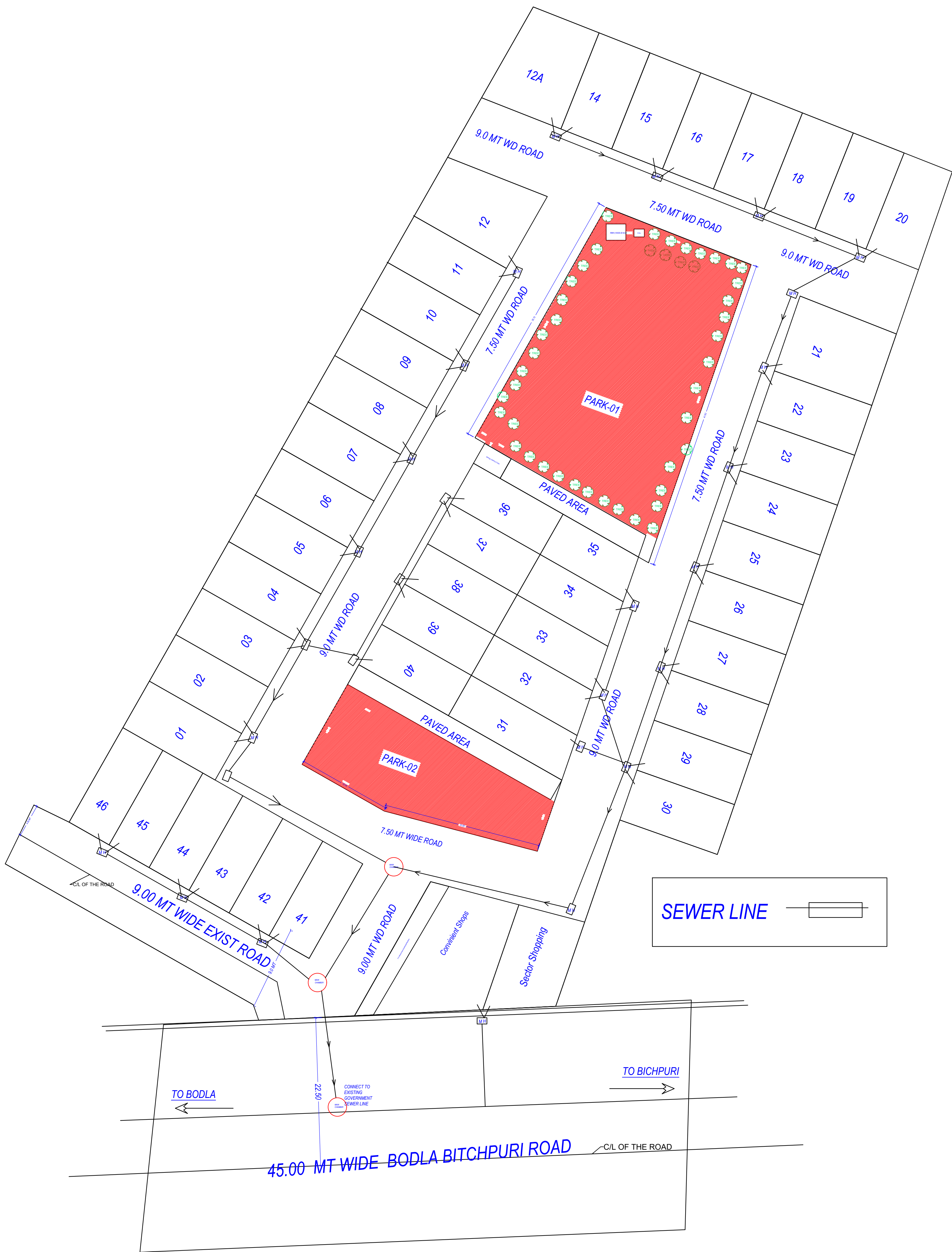
SEWER LINE PLAN
