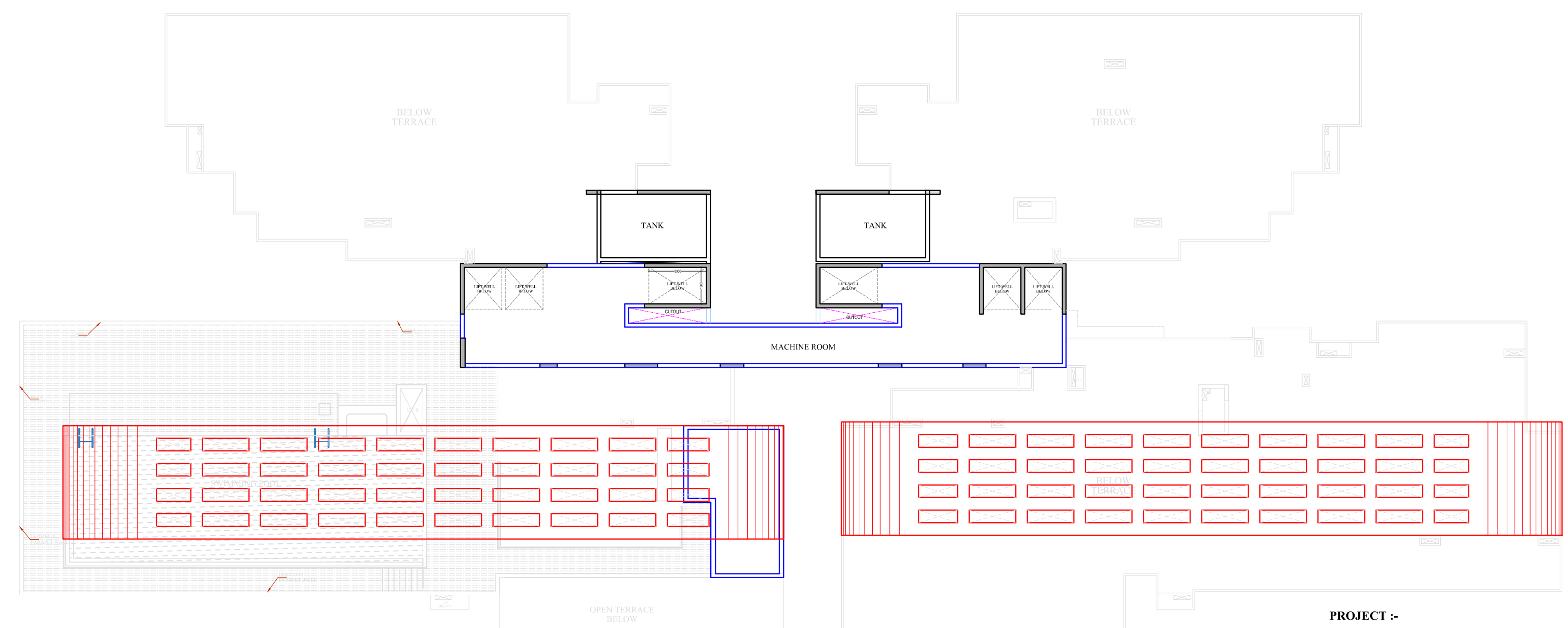
LIFT MACHINE ROOM & WATER TANK PLAN SCALE 1.300
