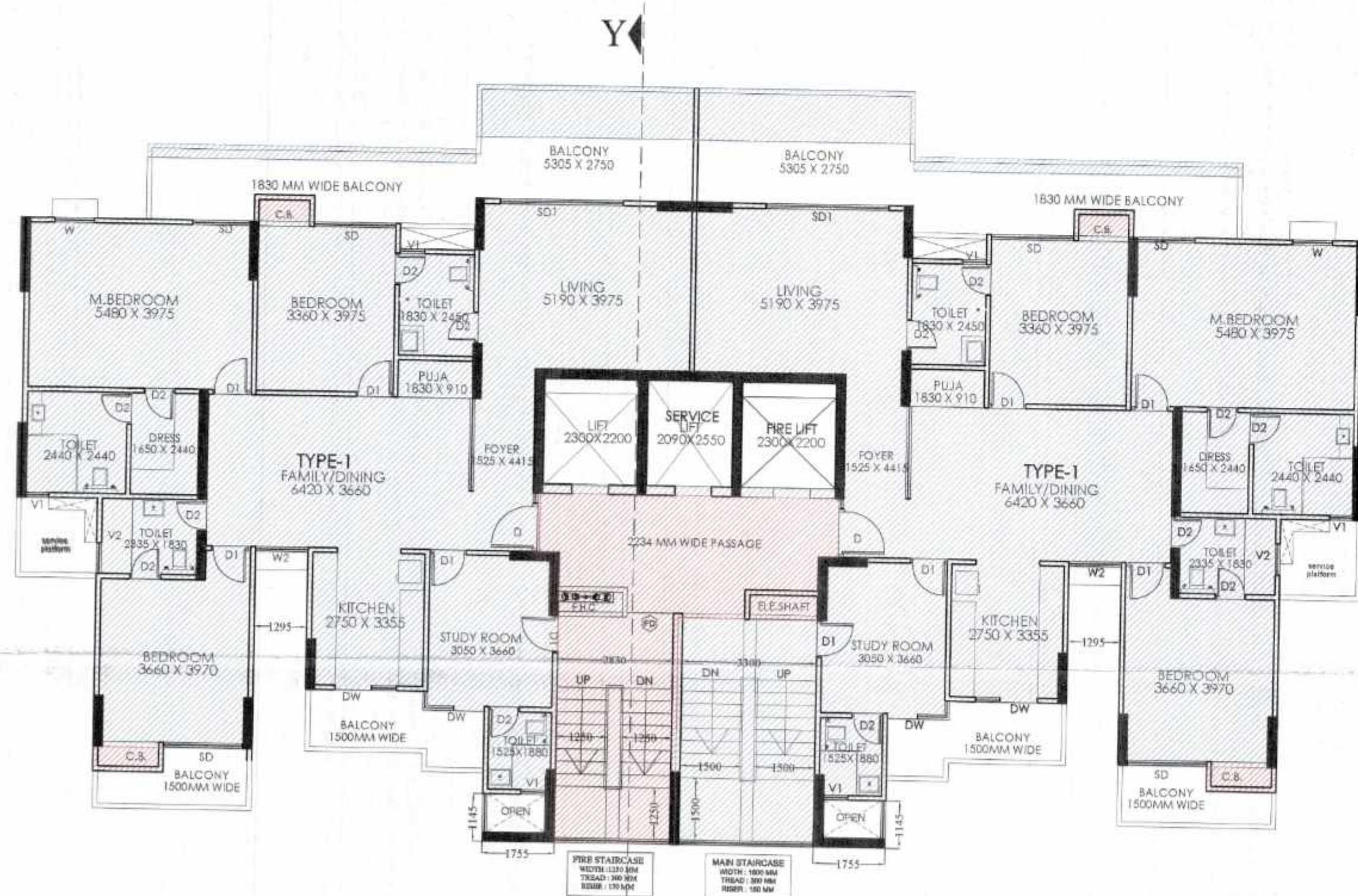
2nd TO 17th FLOOR PLAN & 19th TO 21st FLOOR PLAN
