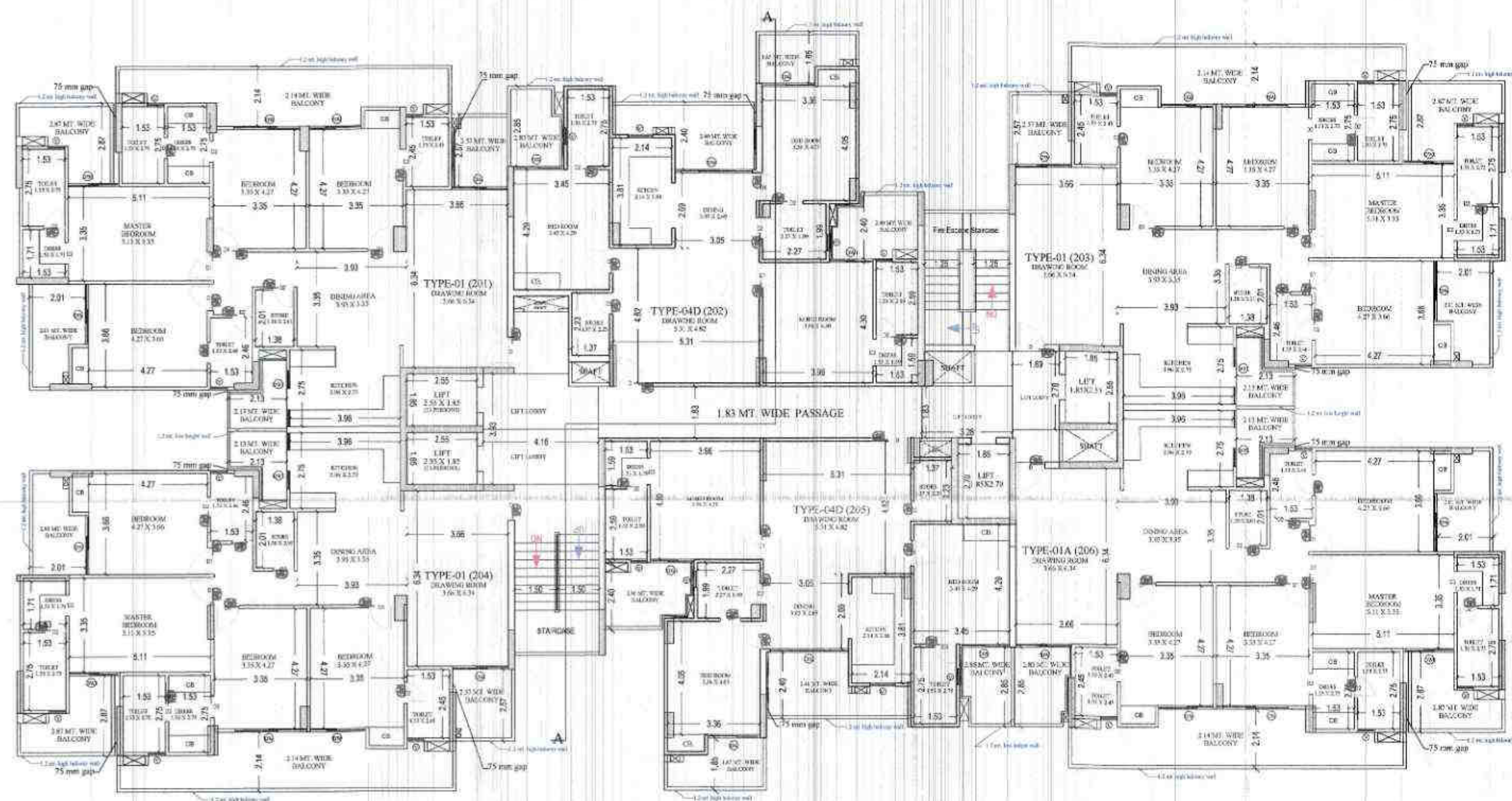
TYPICAL - 2-14 FLOOR PLAN (Proposed) (SCALE 1:100)
