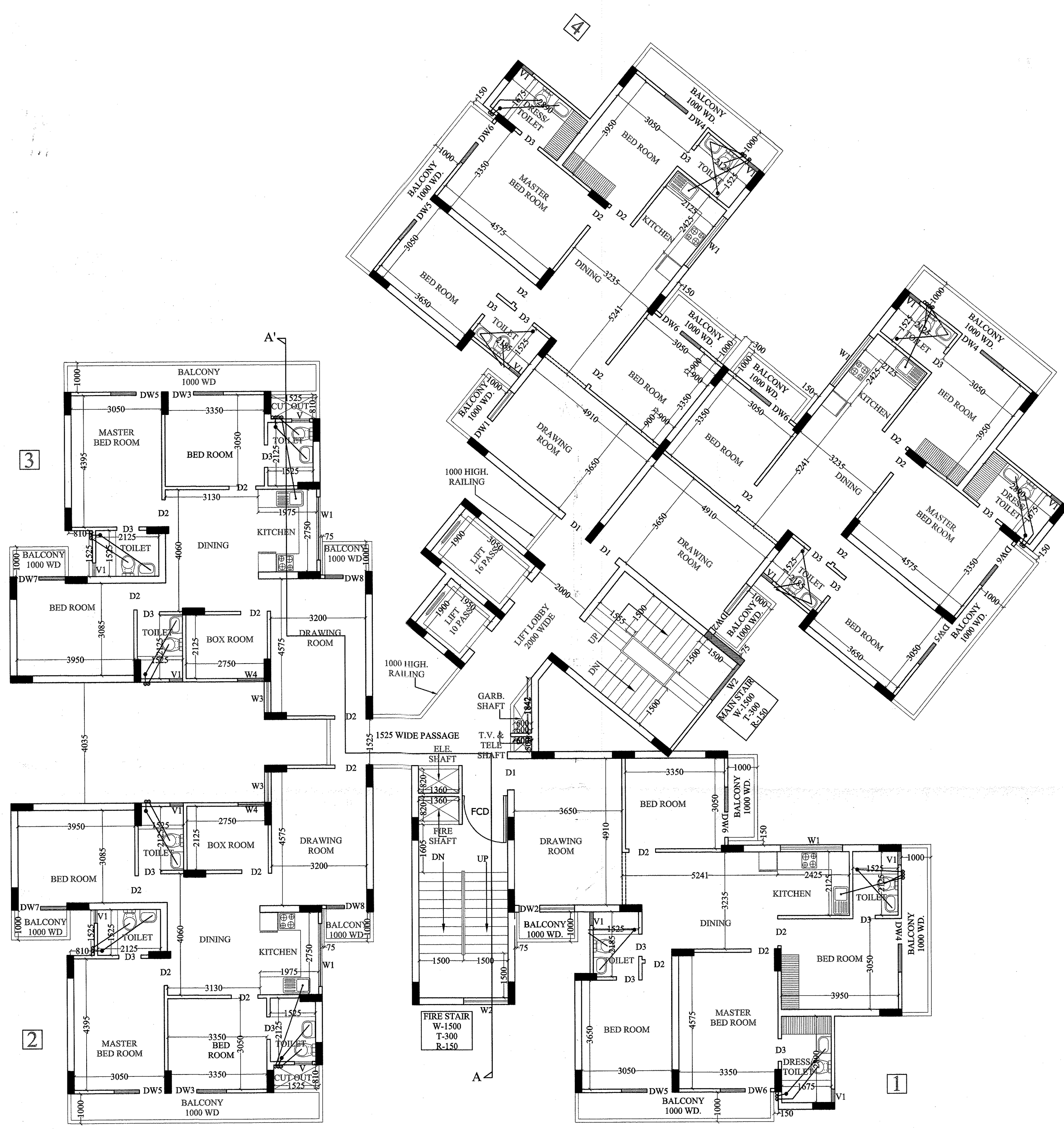
ELEVATION-A TOWER - D1 1st. TO 21st. FLOOR PLAN
