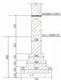
TYP. SECTION FOR 230 THK. BRICK WALL (SCALE=1:20)
