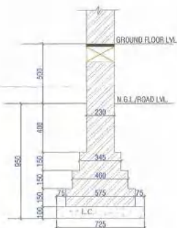
TYP. SECTION FOR 230 THK. BRICK WALL (SCALE=1:20)
