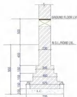
TYP. SECTION FOR 230 THK. BRICK WALL (Scale=1:20)
