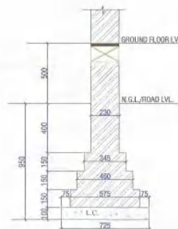
TYP. SECTION FOR 230 THK. BRICK WALL (Scale=1:20)
