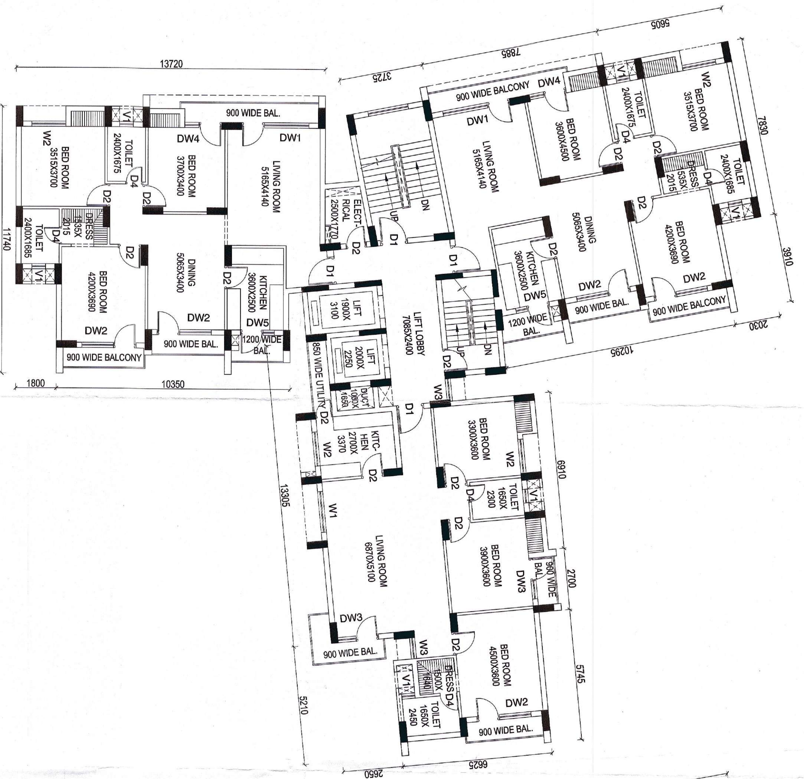
TYPICAL FLOOR PLAN ( BLOCK-N ) (2nd,3rd,13th,14th & 15th Floor) SCALE - 1:100
