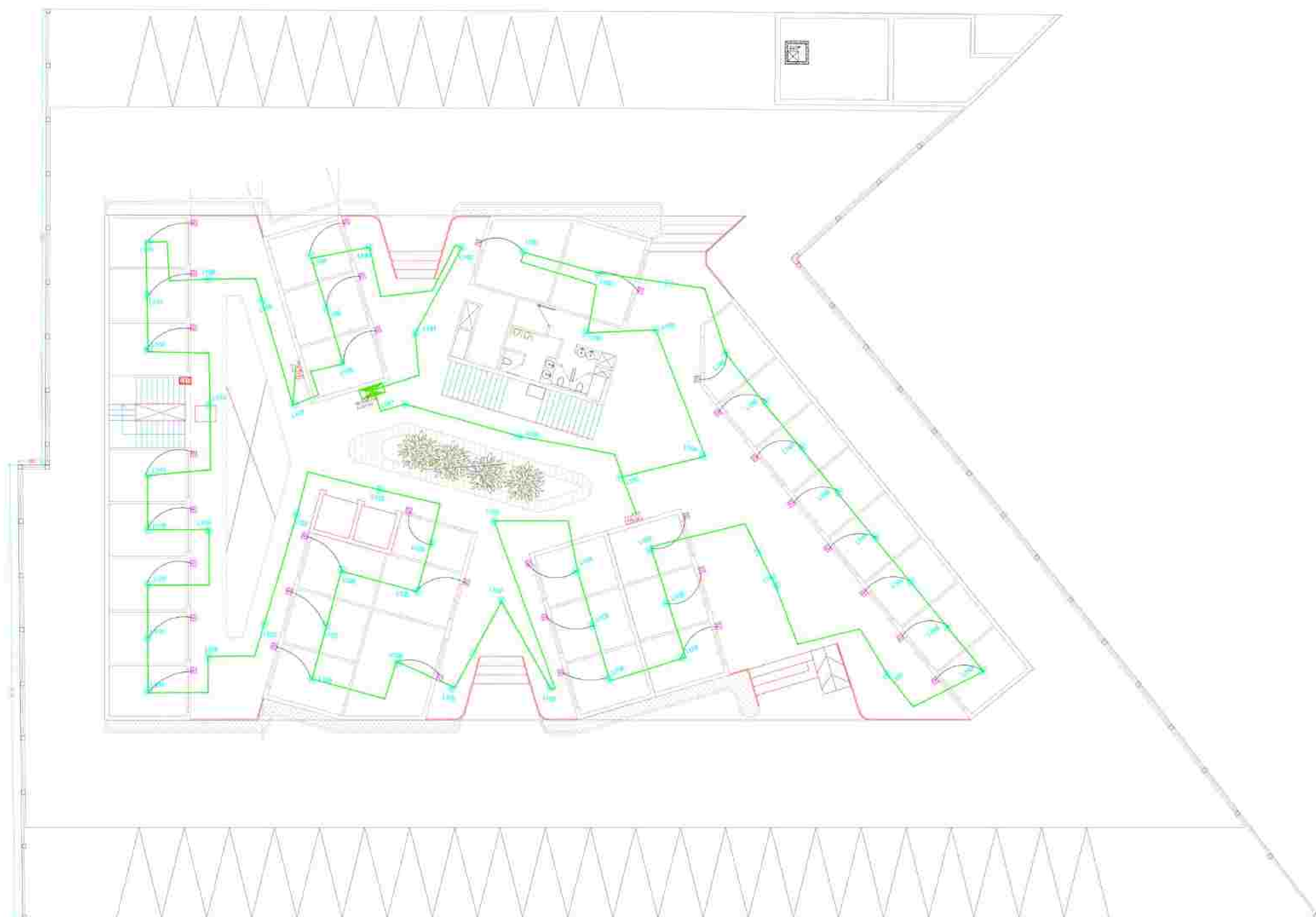
GROUND FLOOR PLAN FIRE ALARM LAYOUT PLAN
