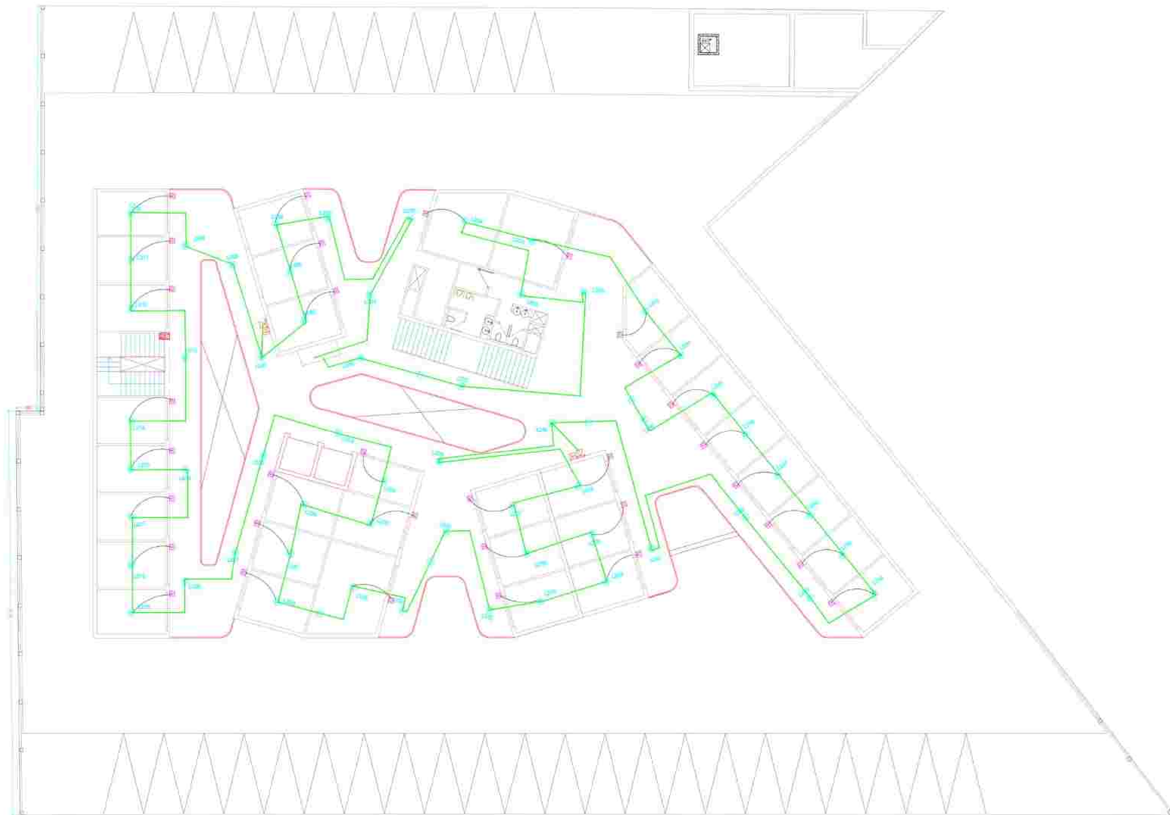
FIRST FLOOR PLAN FIRE ALARM LAYOUT PLAN
