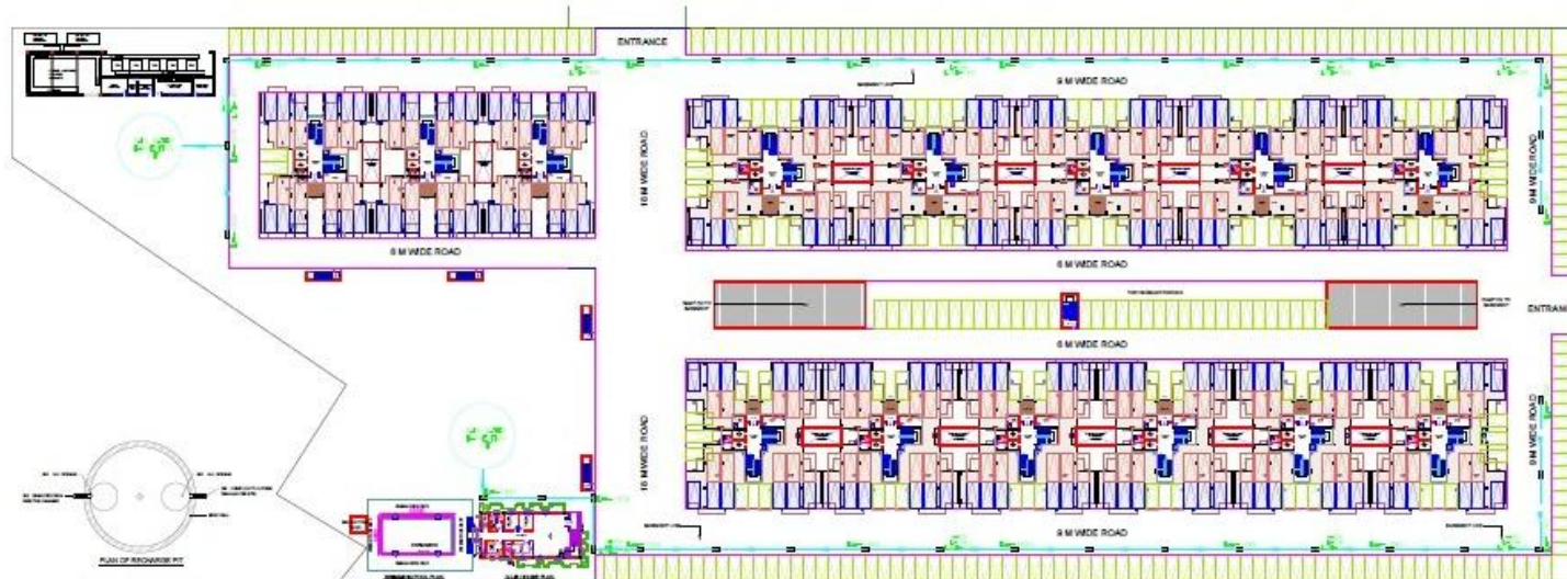
EXTERNAL CATCH BASIN LAYOUT PLAN FOR ENVIROMENTAL CLEARANCE
