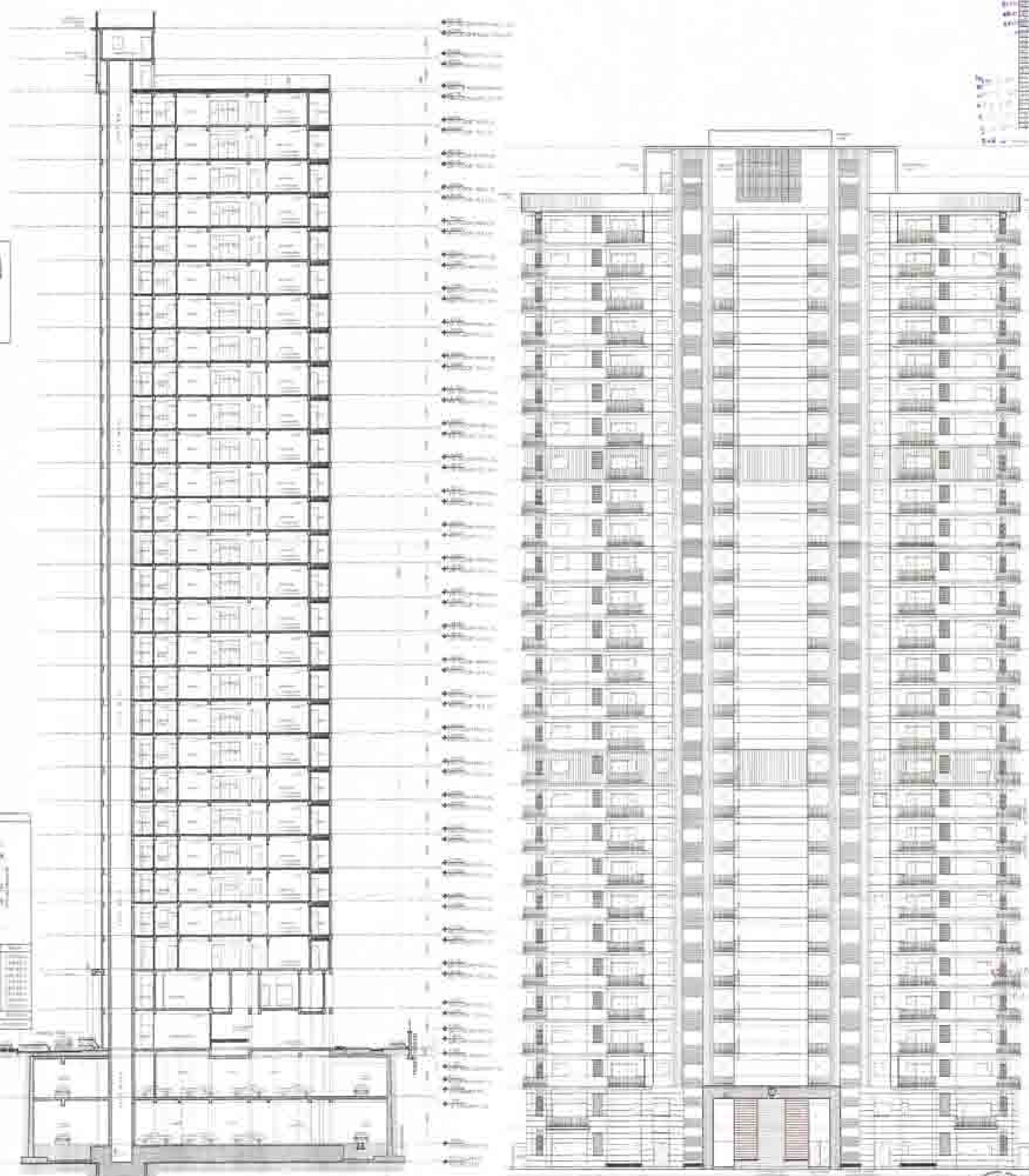
FRONT ELEVATION TOWER 2
