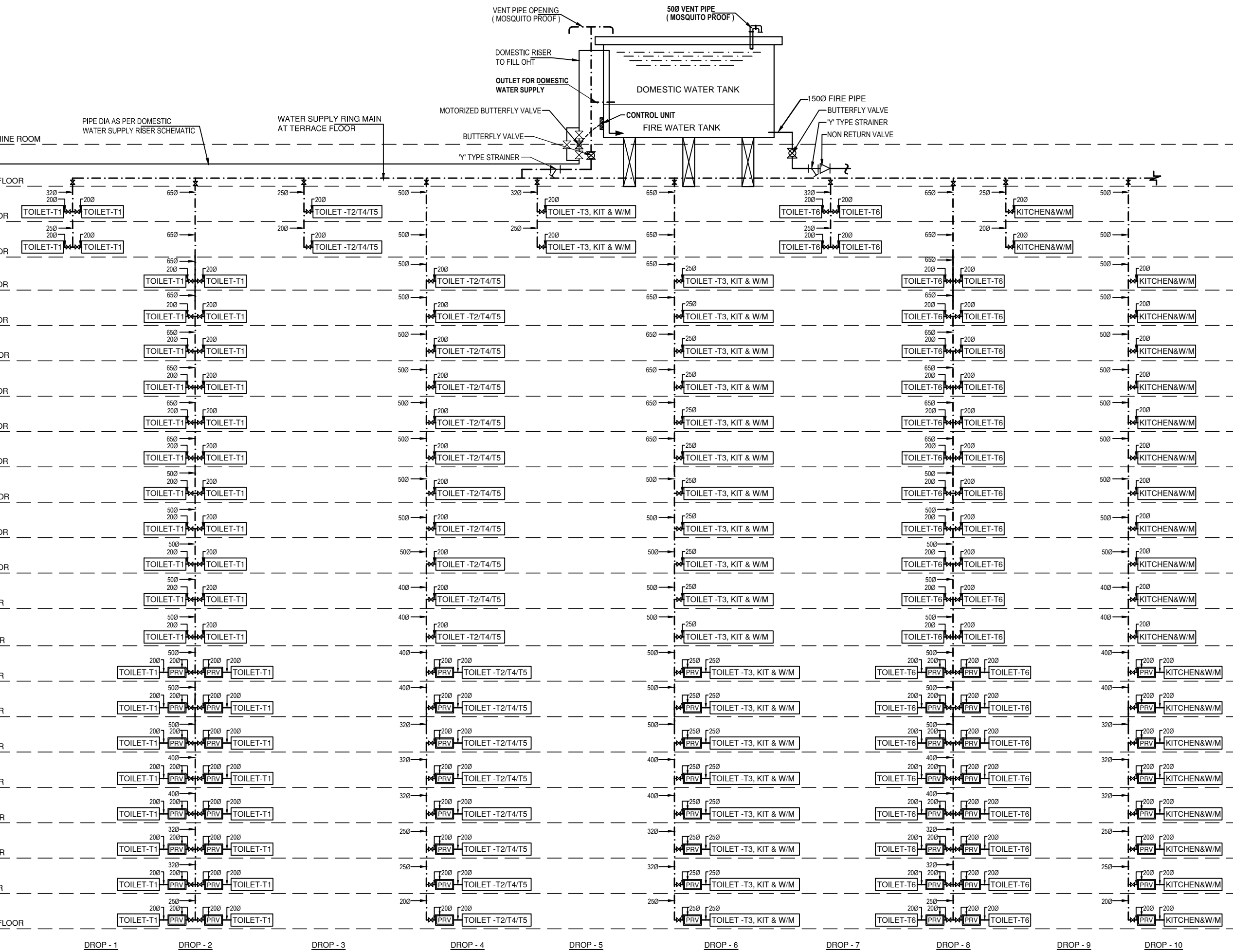
DETAIL OF DOMESTIC WATER SUPPLY DROPS
