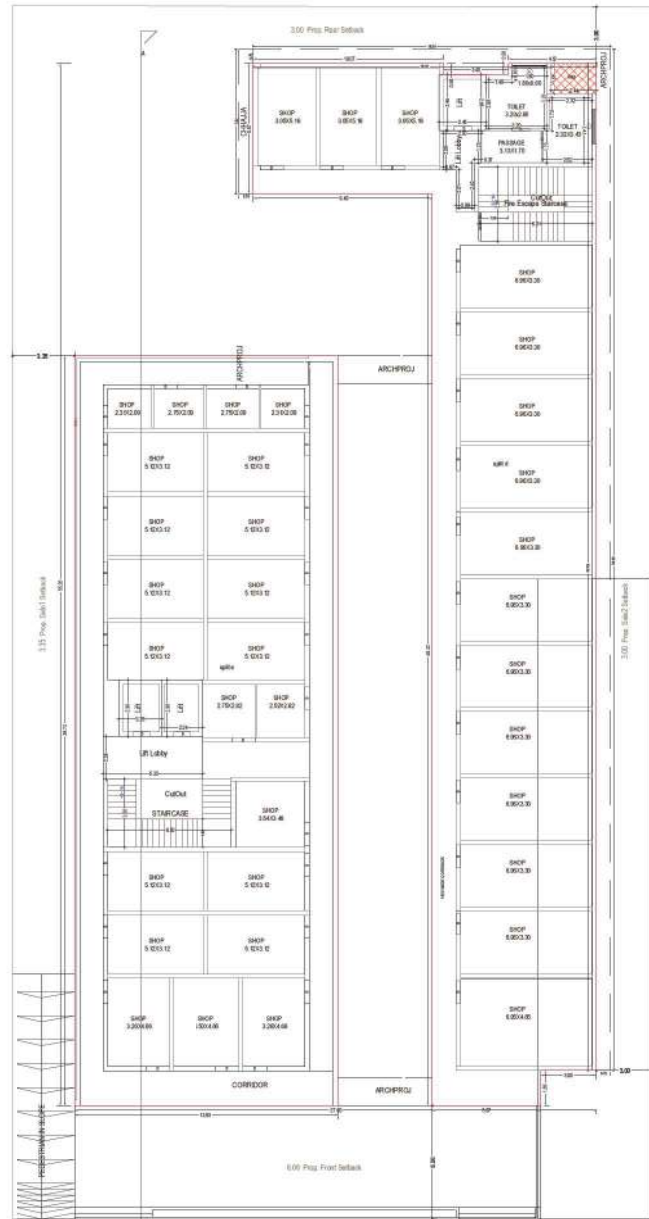
UPPER GROUND FLOOR PLAN (Proposed) (SCALE 1:100)
