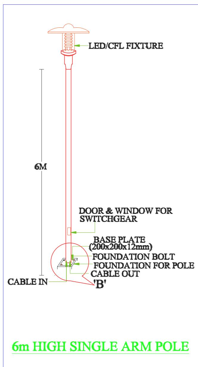
L1 - EXTERIOR 6M HIGH POLE WITH 45W LED ASYMMETRIC FORWARD THROW FIXTURE (IP65 RATED)
