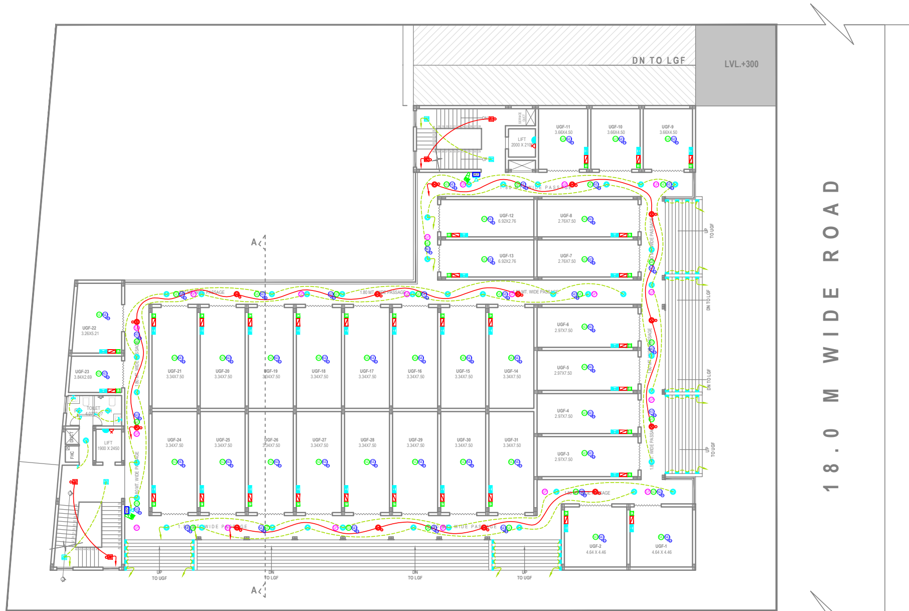
ELECTRICAL -LIGHT & POWER LAYOUT (UPPER GROUND FLOOR PLAN)
