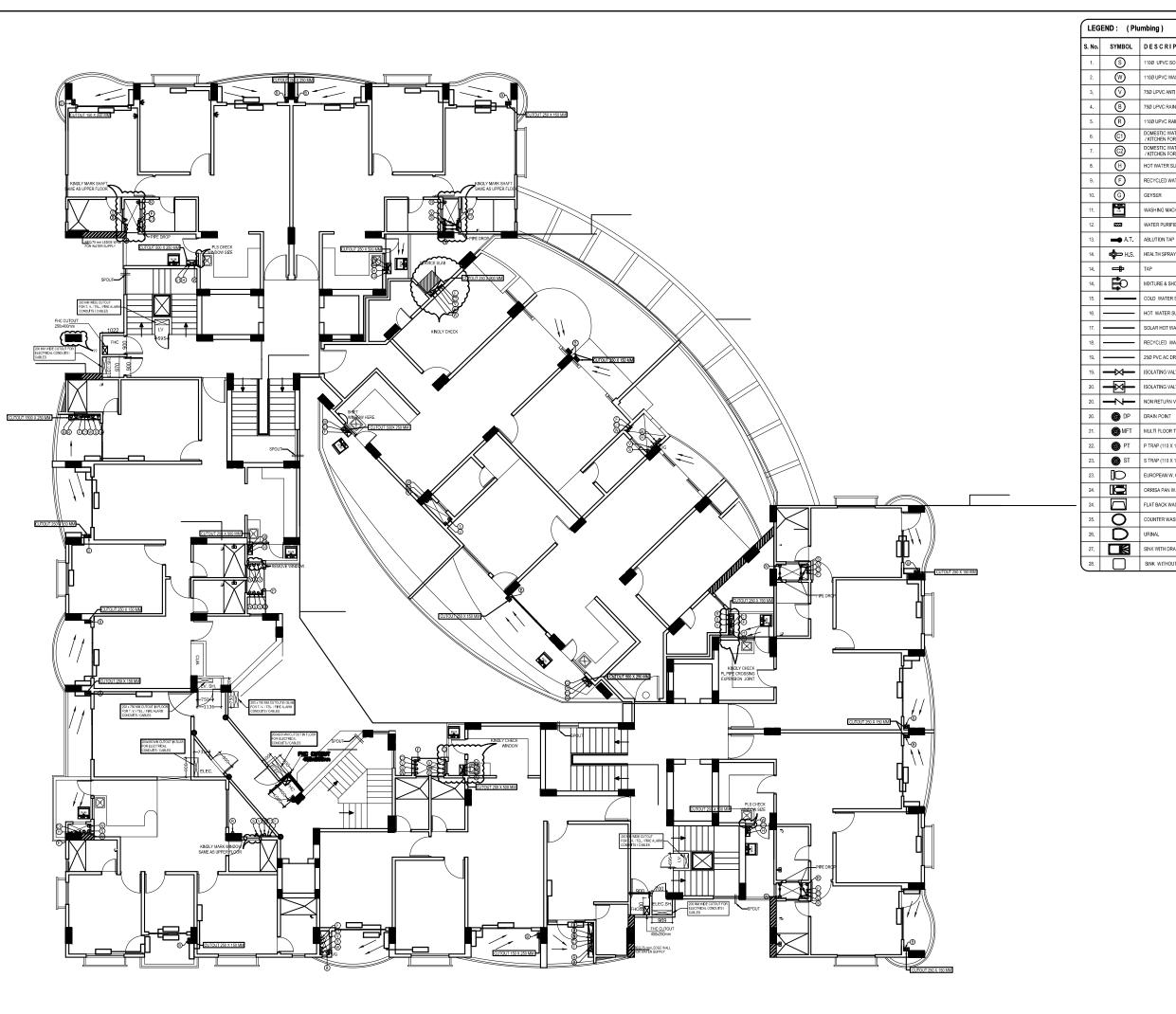
NOTES: (Plumbing) COLD WATER SUPPLY PIPE MATERIAL a) For inside toilet (domestic) - CPVC (SDR-11) with solvent DESCRIPTION UPVC SCH 40 Pipes With SCH 80 fittings by solvent cement joint 110Ø UPVC SOIL AND VENT PIPE UPVC SCH 80 Pipes With SCH 80 fittings by solvent cement joint 110Ø UPVC WASTE AND VENT PIPE G. I. ( CLASS B ) by teflon tape
